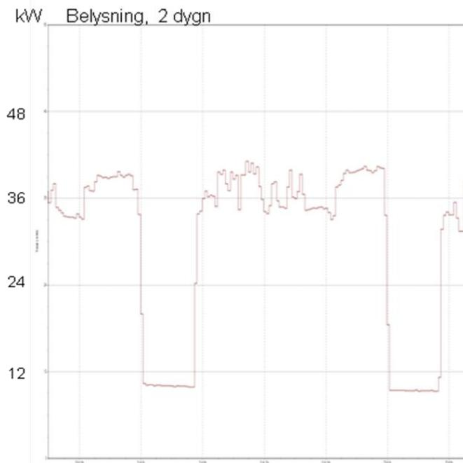
**Figure 5. Energy used for lighting during 48 hours.**
