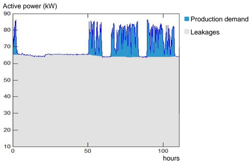
**Figure 1.** Example of measured electricity use for compressor (90 kW). The measurements started Friday afternoon and show the consumed power during the weekend and beginning of the week.
